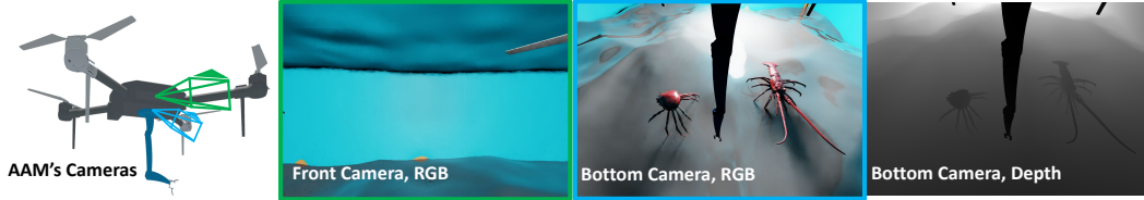
Figure 9: Camera positions (red, green, and blue arrows are X, Y, and Z axes, respectively) and views of the cameras
