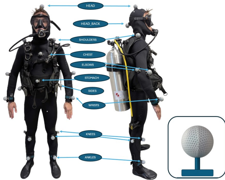
Fig. 3: Diver equipped with a 19-marker custom set (30mm and 40mm diameter markers) for use with the Qualisys motion capture system. Example of a marker depicted in the bottom right of the Figure.
