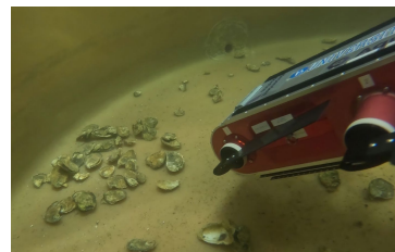
A hexapedal robot with edging computing on board, detecting oysters. Image from Xiaomin.
