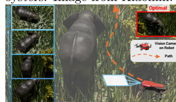
A drone selecting the optimal viewpoint[10] for object detection. The images are best seen in color on a computer screen at 400% zoom. Image from Xiaomin.
